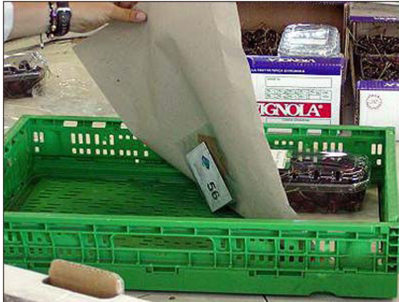
RFID temperature tags were mounted between boxes of cherries and reusable containers, as well as underneath sheets of paper (shown here).
